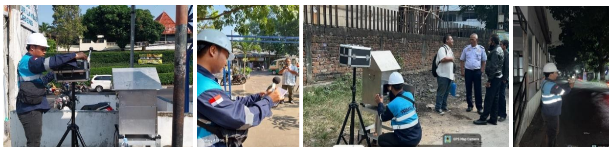
Ambient air quality measurement using a High-Volume Sampler (HVS) and noise level measurement using a Sound Level Meter by KAN-accredited independent laboratory personnel
