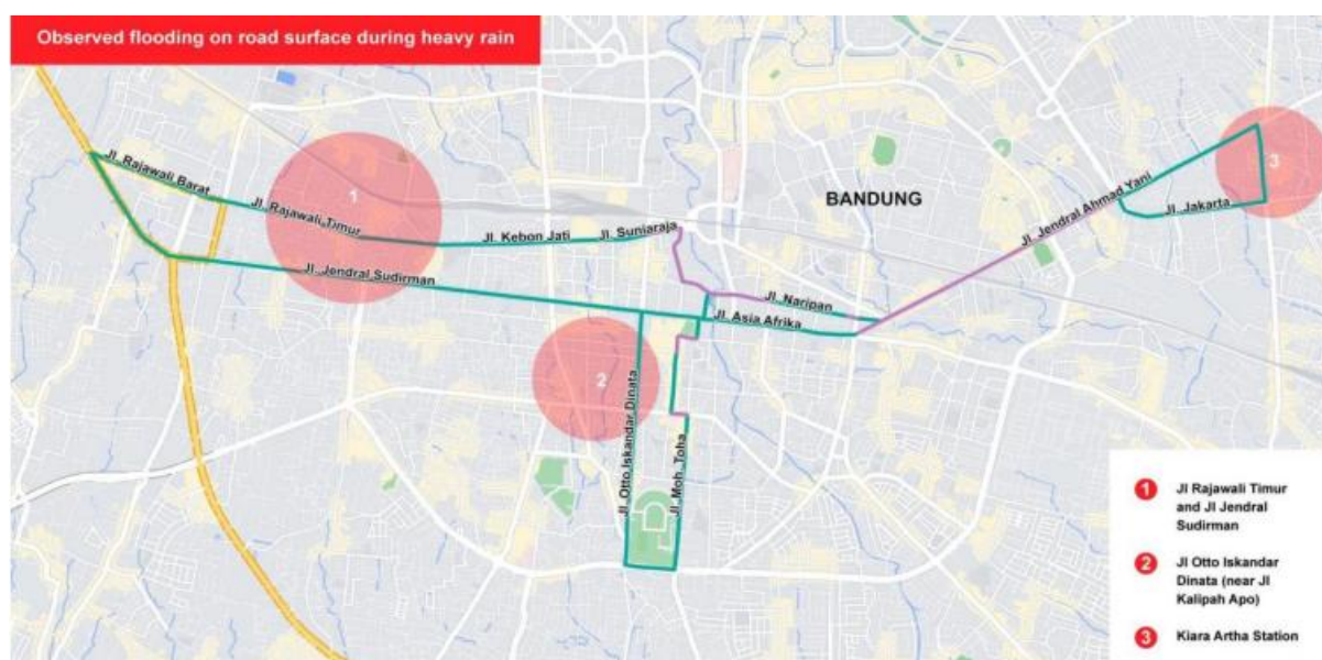
Figure 25. Flooding and Water Puddles Sites within BRT On-corridor
